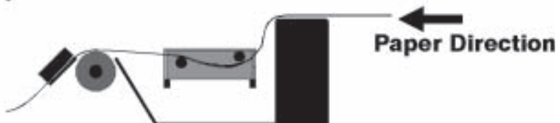
Figure 3- 7. Fanfold guide path
